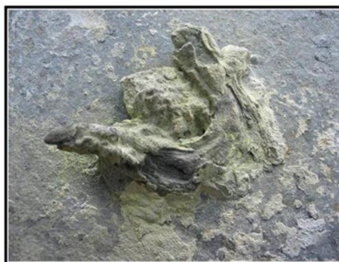
Figure 6. Remnant of Metallic Anchor Exhibiting Sulfide Attack
