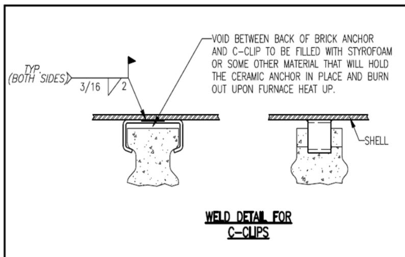
Figure 12. Weld Detail for C-Clips Showing Void Between Brick and Clip
