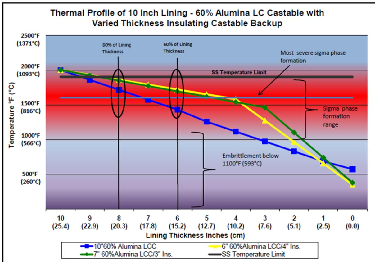
Figure 7. Thermal Profile of Refractory Linings Illustrating Internal Refractory Temperatures
