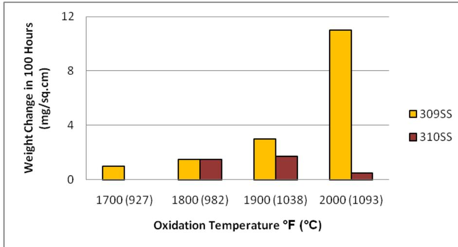
Figure 3. Oxidation of 309 SS and 310 SS Measured by Weight Change
