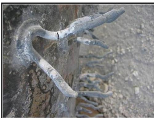
Figure 5. Metallic Anchor Exhibiting Sulfide Crack and Embrittlement
