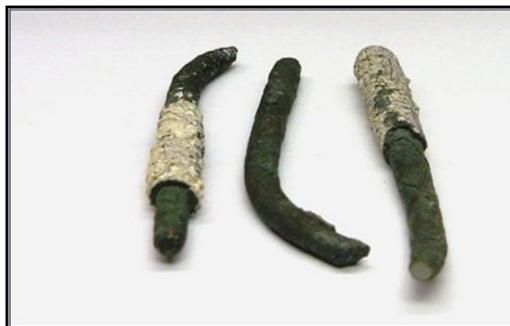
Figure 4. Chromic Oxide Scale and Sigma Phase.
